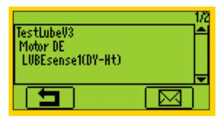
If Dynamic measurement is chosen, your SDT270DU LUBExpert will automatically collect Dynamic data from your initial and final reading. The process is entirely the same as described before with difference that you will be providing additional highly valuable data for bearing Condition Monitoring.
