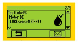
Next position in your work order/survey is Static data measurement of the same asset. Since data has been collected and lubrication task performed, this position is clearly marked as "Done" and you can proceed to your next asset.
