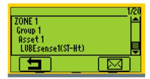
At this point, a message icon is offered in the lower right corner of the display. If the asset is not in operation, or safety is compromised, you have an option to assign a message that explains these conditions and your decision to abort the planned work.
