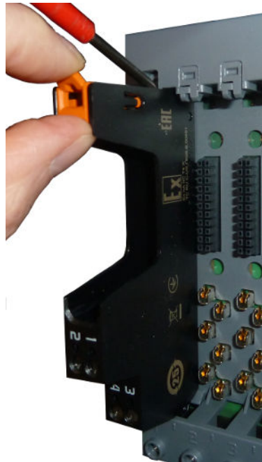
Figure 6-2: Remove a Terminal Block
