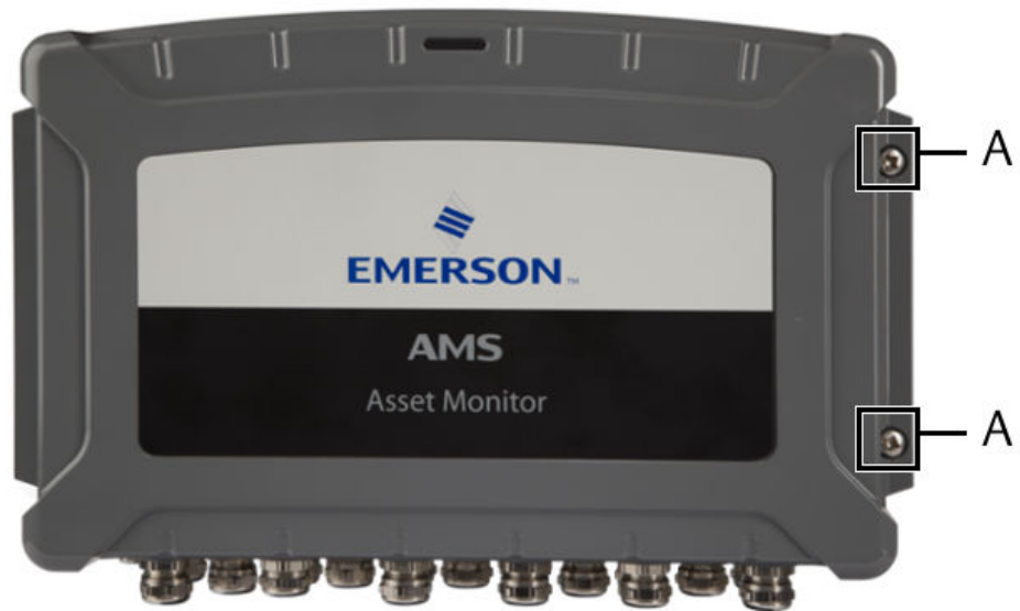
Figure 4-7: Position of the screws
